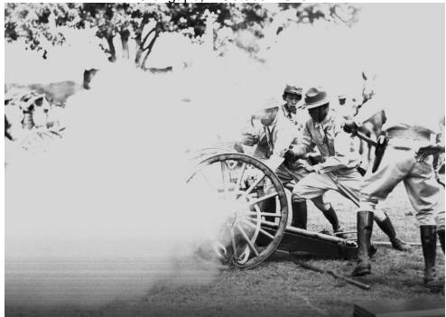
October 1940 at Olongapo: Cannoneers of the 23<sup>rd</sup> Field Artillery(PS) fire the 2.95" Vickers-Maxim mountain gun. The 830 pound gun which could be broken down into four pack mule loads could hurl a 12.5 pound shell to a range of 4,825 yards.
